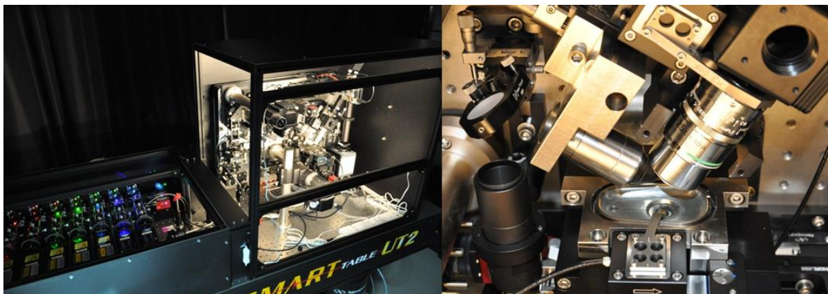
Clone of Eric Betzig's LLSM in iBiOs. The LLSM is equipped with seven lasers (405 nm, 445 nm, 488 nm, 532 nm, 561 nm, 589 nm, 642 nm) and a live cell periphery for fast volumetric imaging with single molecule sensitivity.
